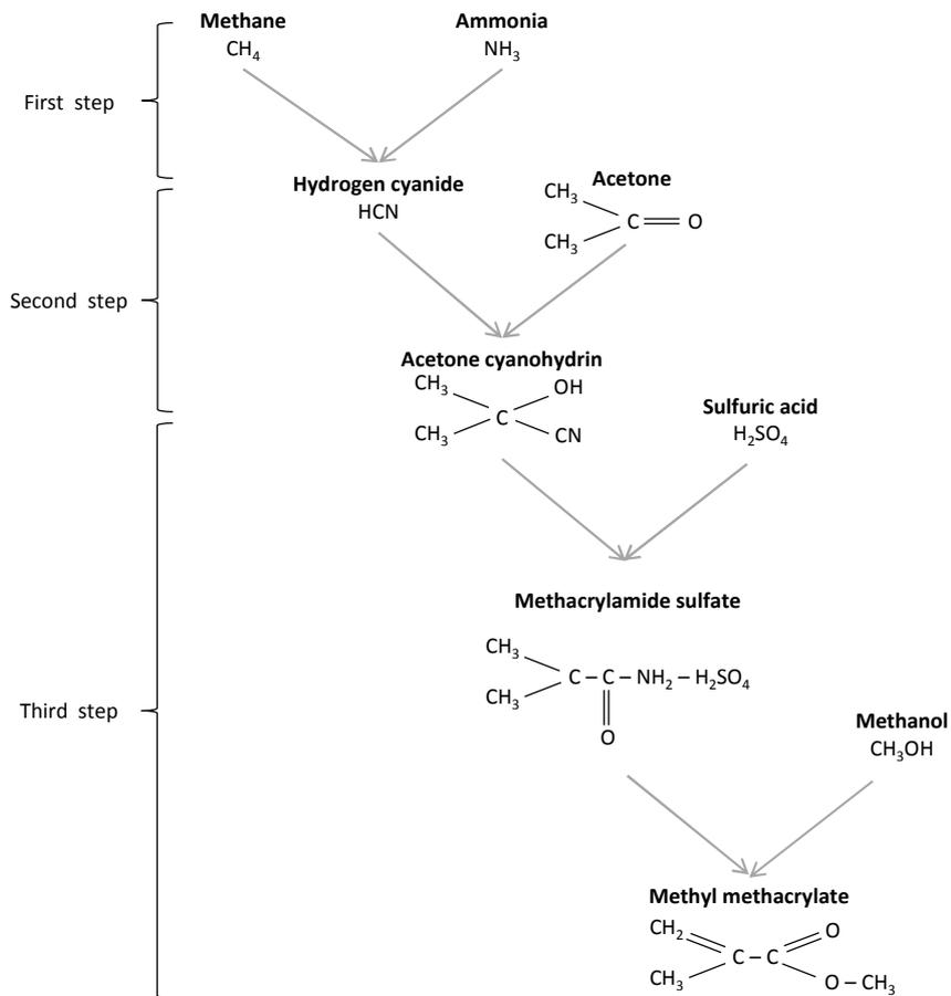
Figure 2: MMA production process
